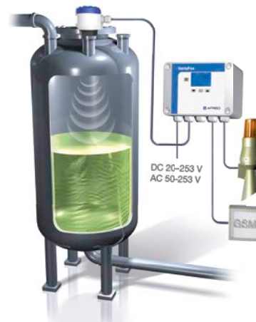
Non-contact level measurement with ultrasonic measuring instrument UST 20 and digital display unit VarioFox® 24 as stand-alone complete solution for individual tanks and small tank farms.
