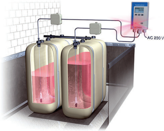
Fig. 6: Level measurement with detection of difference at battery tanks
