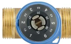
The new series ATM thermal mixing valves excel with extremely simple handling: The fitter can rapidly adjust the desired temperature of the mixed water in °C by means of the dual scale; later on, only the adjusted scale value (1–6) is visible through the window in the cap. If space is limited and the control knob cannot be used, adjustments can also be made via the integrated 7 mm hexagon socket. In addition, the cap can be lead-sealed to the mixing valve to help prevent unwanted adjustments.
