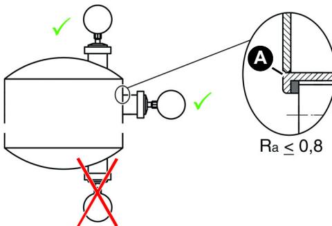
1. Parts welded to the tank must be mounted flush with the inside wall of the tank (A).
