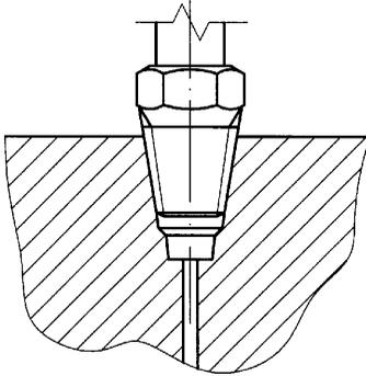
*Fig. 6: Conical threads, sealing in the thread*
