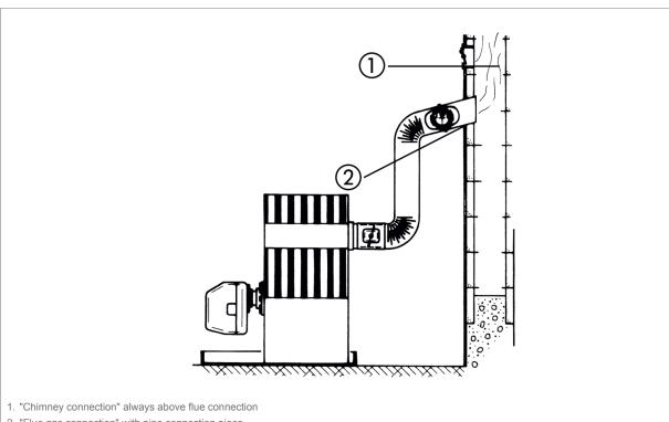
2. "Flue gas connection" with pipe connection piece
