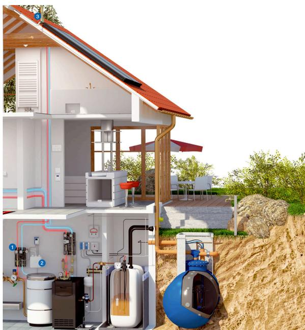
1. Solar pump assembly PrimoSol® 130-4
