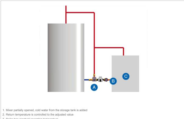
3. Boiler has reached operating temperature
